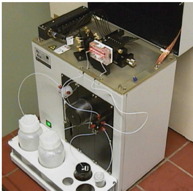
Fig. 1. Prototype set-up of the optical immunosensor RIANA (river analyzer). A FIA system delivers sample, buffer and regeneration solutions to the flow-cell, where a transducer is mounted. Laser light excites the fluorescently labeled antibodies involved in the immunoreaction taking place over the transducer. Fluorescent light is detected by photodiodes and acquired by lock-in detection.
